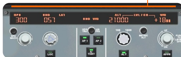
Figure 39 – FCU CRZ altitude and SPD selected
