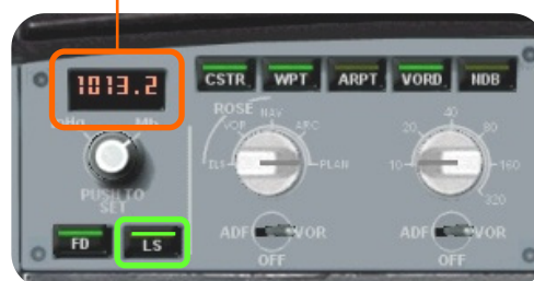
Figure 58 – EFIS Control Panel
