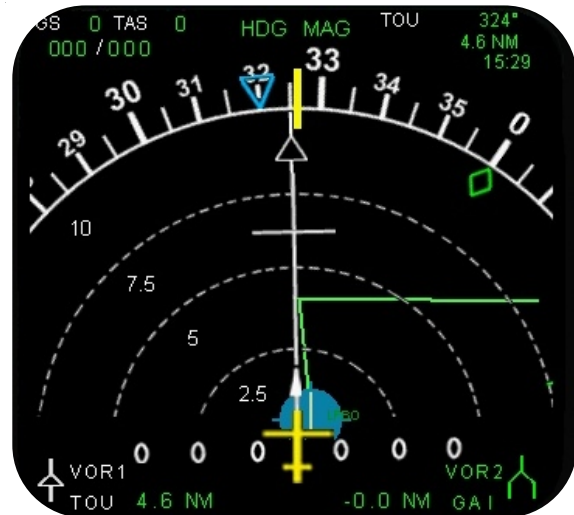
Figure 24 – ND ROSE Selector in the ARC Mode
