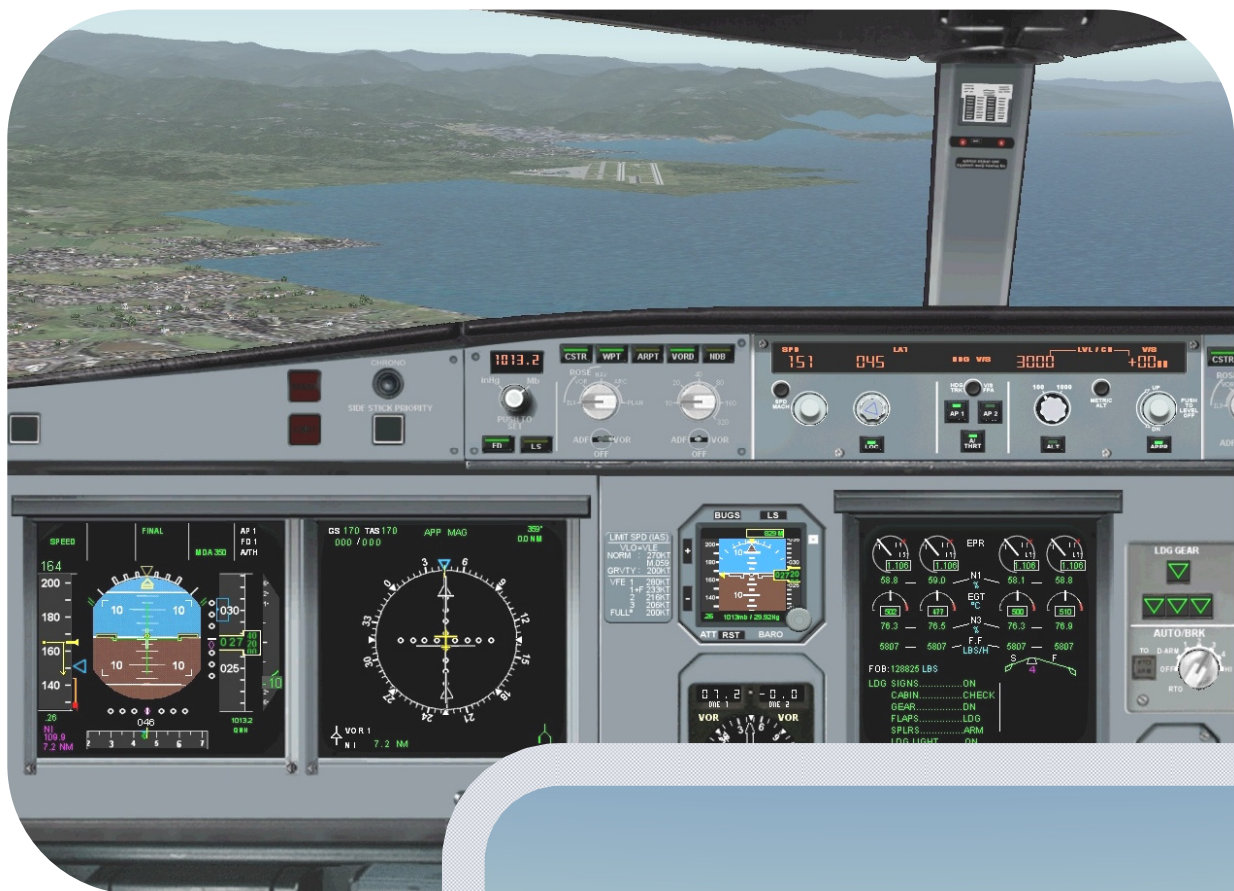
Figure 61 – Cockpit Overview/PFD LOC and GS alive
