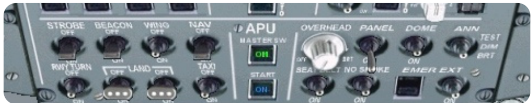
Figure 28 – Overhead Panel / LIGHTS/APU Part
