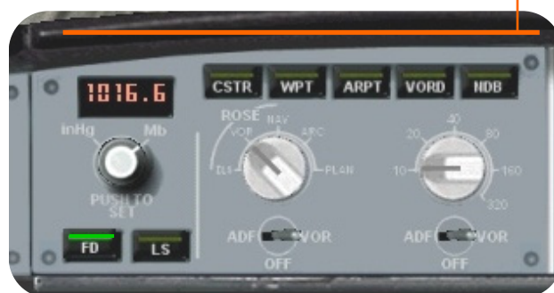
Figure 15 – FCU – EFIS Control Panel
