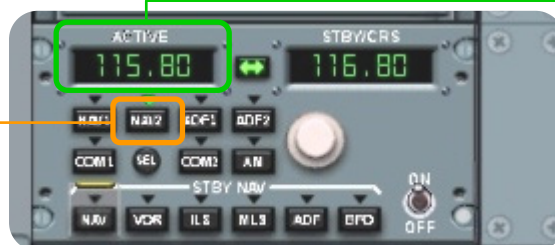
Figure 19 – RMP NAV2 with GAI VOR frequency
