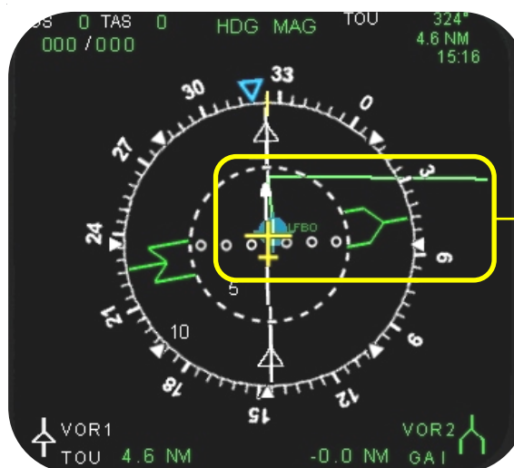
Figure 23 – ND ROSE Selector in the NAV Mode
