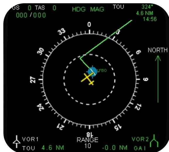
Figure 25 – ND ROSE Selector in the PLAN Mode
