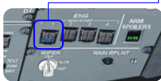
Figure 31 – Overhead / ENG MAN START Panel
