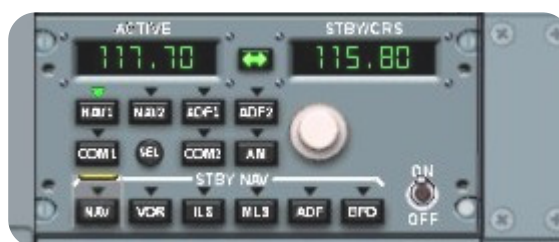
Figure 18 – RMP NAV1 with TOU and GAI VOR frequencies
