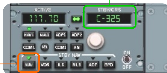
Figure 20 – RMP STBY NAV with TOU CRS
