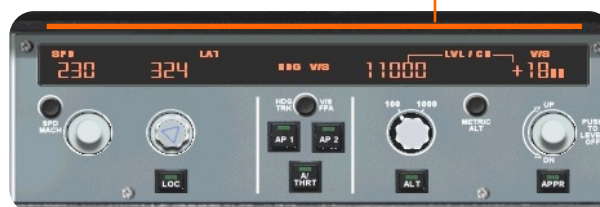
Figure 16 – FCU - Auto Flight System part
