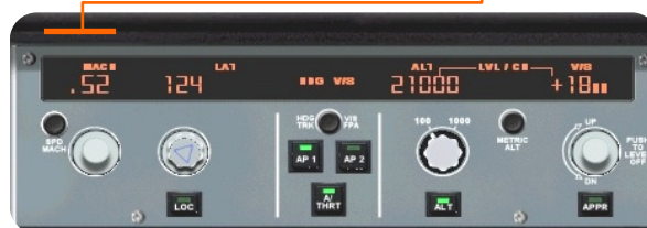
Figure 41 – FCU - AFS Control Panel Mach value
