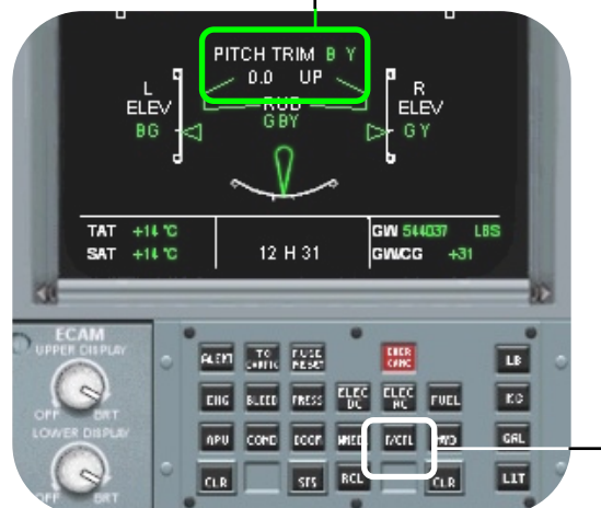
Figure 17 – ECAM Control Panel with LWR ECAM display
